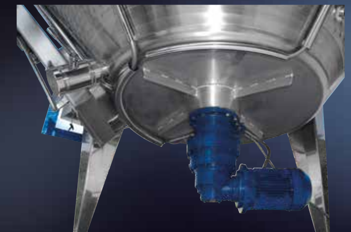
"S" series 1200 hl Meccanotank fermentation tank with cone with extraction blade and Turbotank
