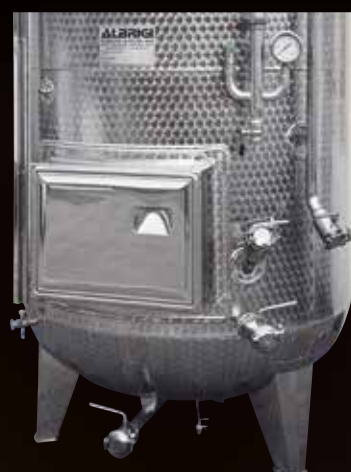
Frigotank with set of total or partial drain valves, Mobilmix removable stirrer and CO2 bottom injector
