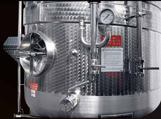
Safety unit with PED calibrated valve
