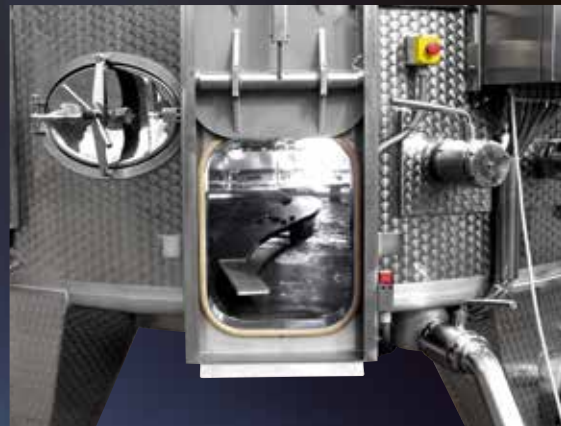
Guillotine door with inside view of the extraction blade
