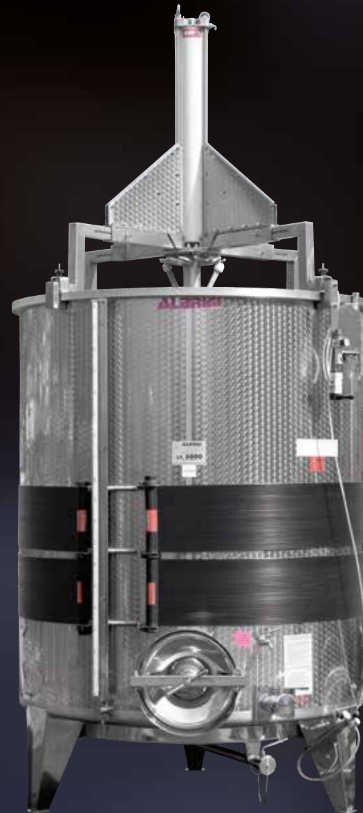
Inside and outside view of the "Variofolltank" punch down mechanism on a 50 hl "Semprepieno" (always full) tank
