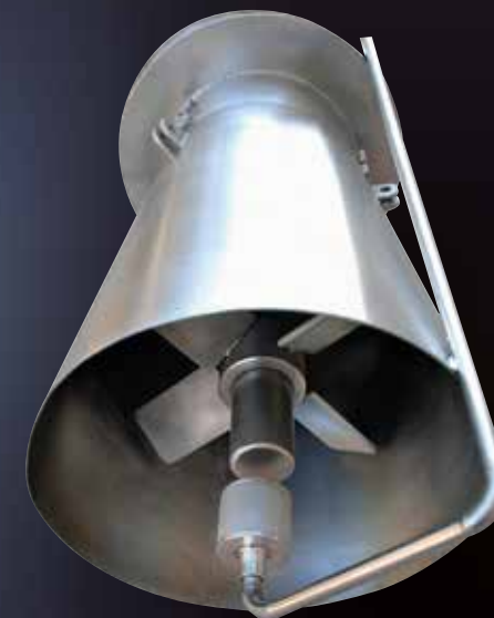
Lower part of the turbine with porous oxygen injection core
