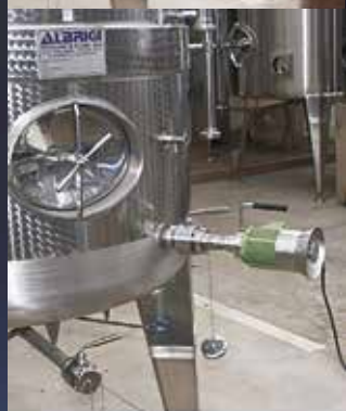
Installation of a Mobilmix mobile removable stirrer mounted on the partial drain valve
