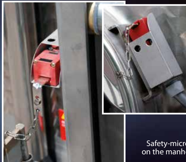
Safety microswitch on the hatchway
