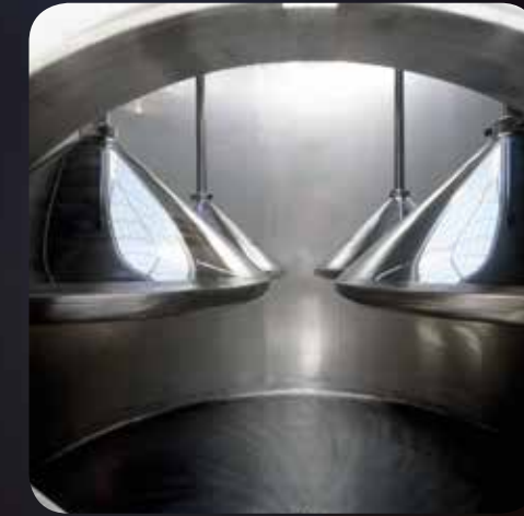
Inside side view of the special self-cleaning pneumatic punching down feet that cover 75% of the surface area of the fermentation tank
