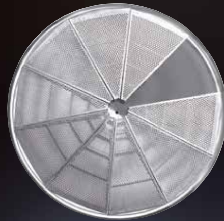
Overhead view of the mobile grate mechanism set on the bottom to keep the whole grapes separated from the must
