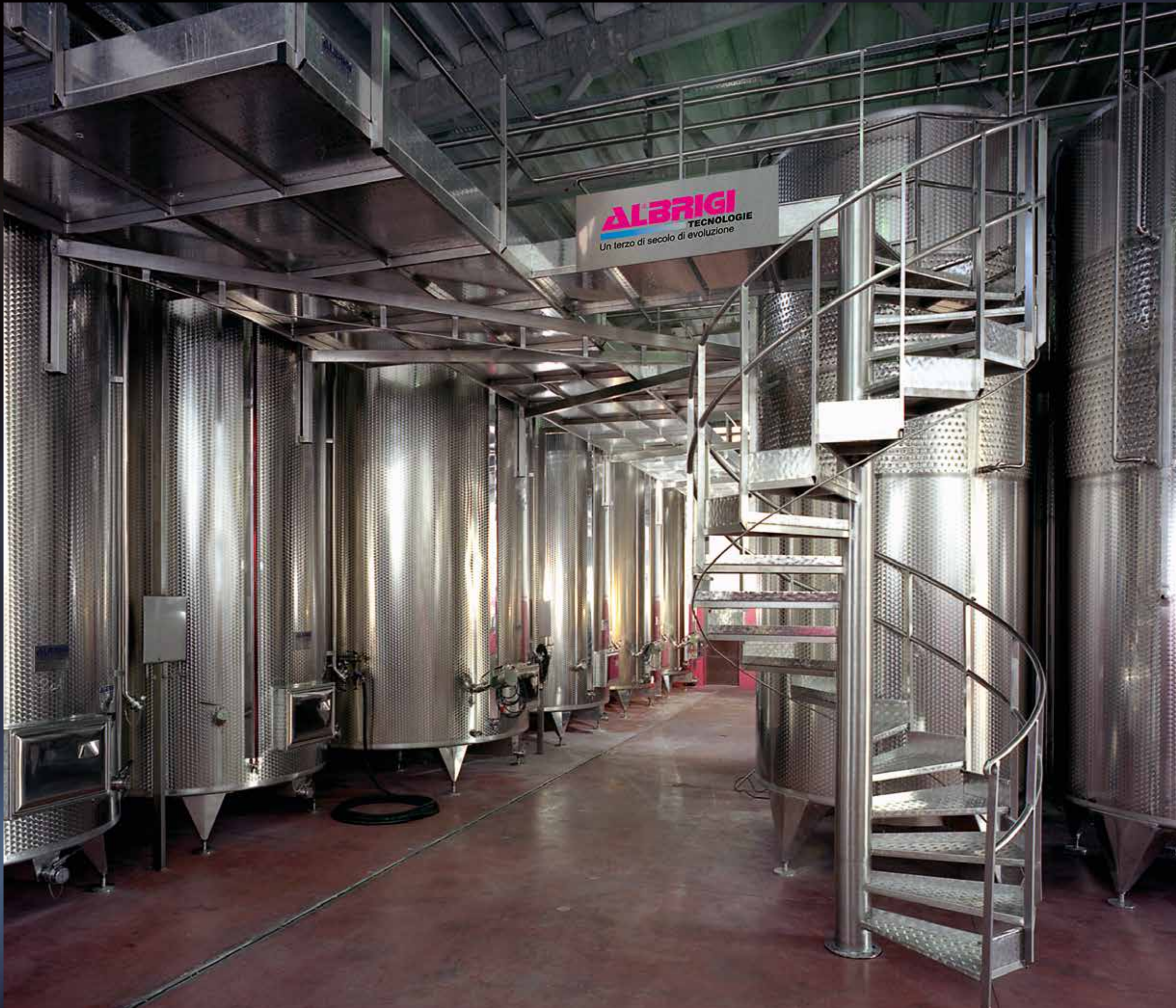
300 and 100 hl Frigotanks, temperature-controlled by Termostar, Isotank insulation, 300 and 150 hl Termotanks, temperature-controlled by Termostar and Cleanfix washing plant
