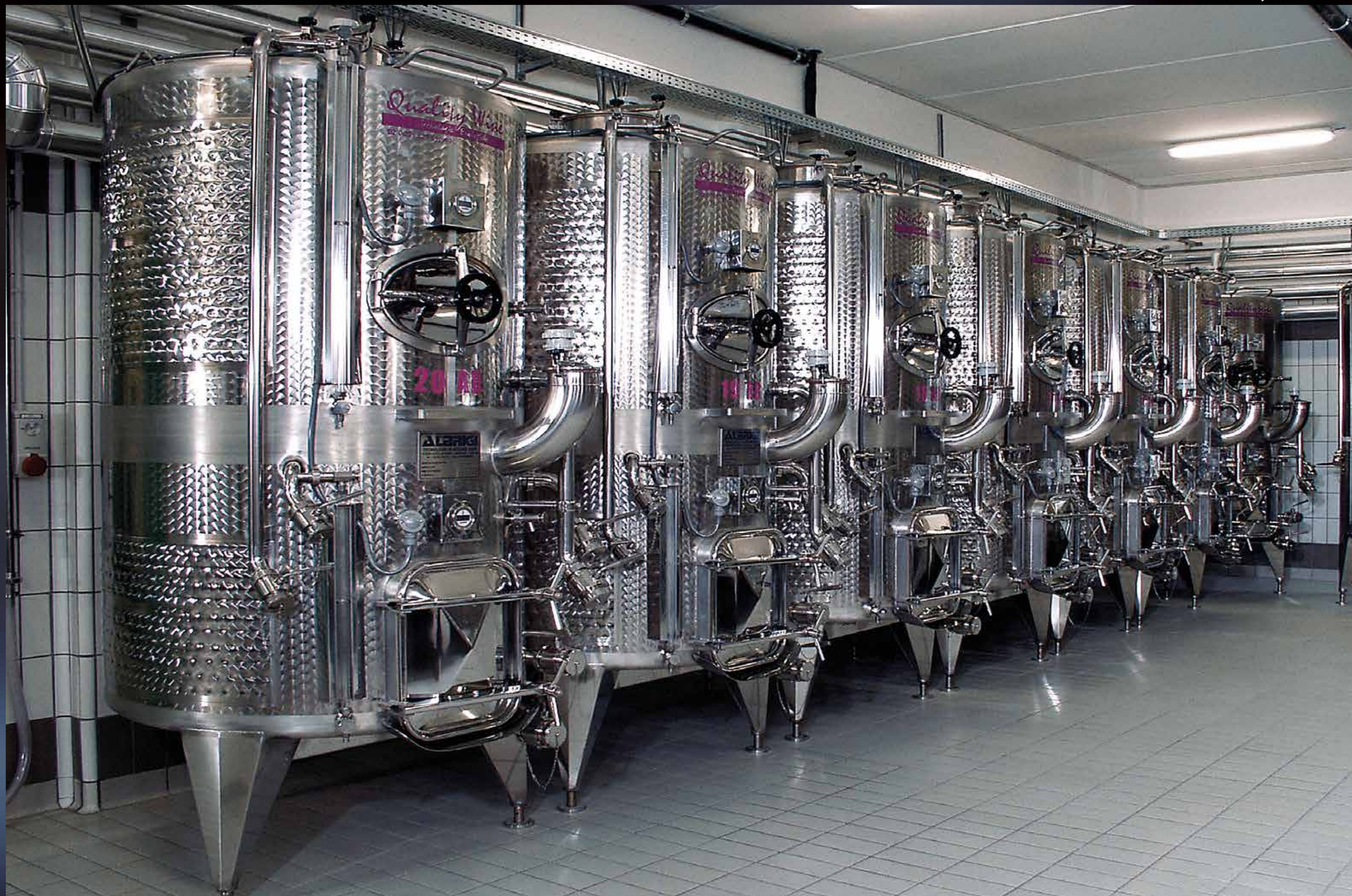
10 + 15 hl Politank Termo with lower fermenting compartment and upper storage compartment, temperature-controlled by Termostar and equipped with Cleanfix washing plant
