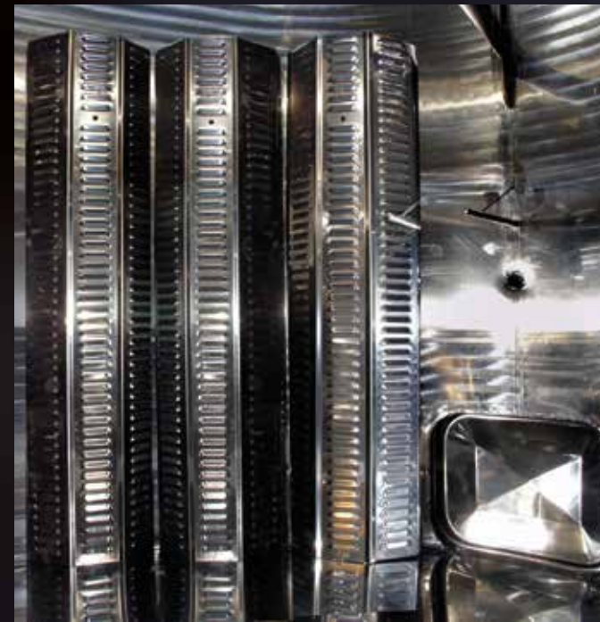
Drain grates to separate must from marc
