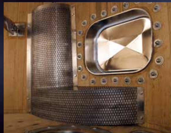
Draining grates mounted on the total drain valve on wooden vats
