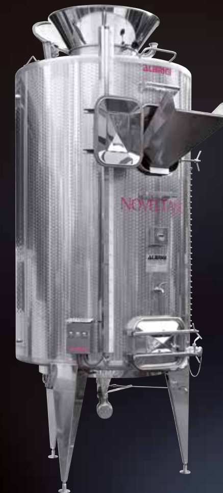
Noveltank with the 2 hoppers for loading the whole grapes
