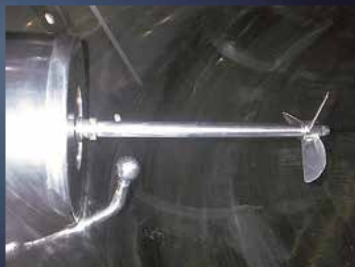
"Sprayball" washing ball for stirrer and mechanical seal cleaning
