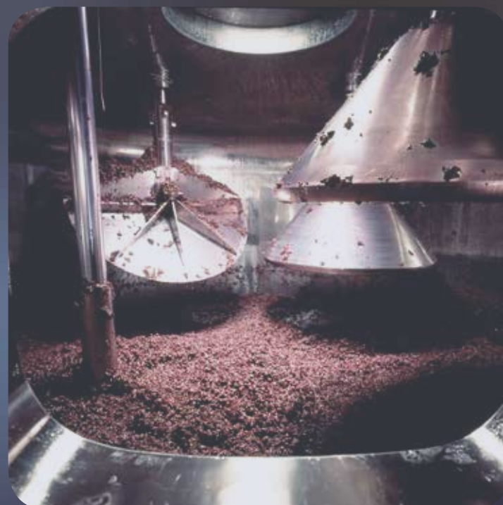
Inside view during punching down with 4 pneumatic feet at work
