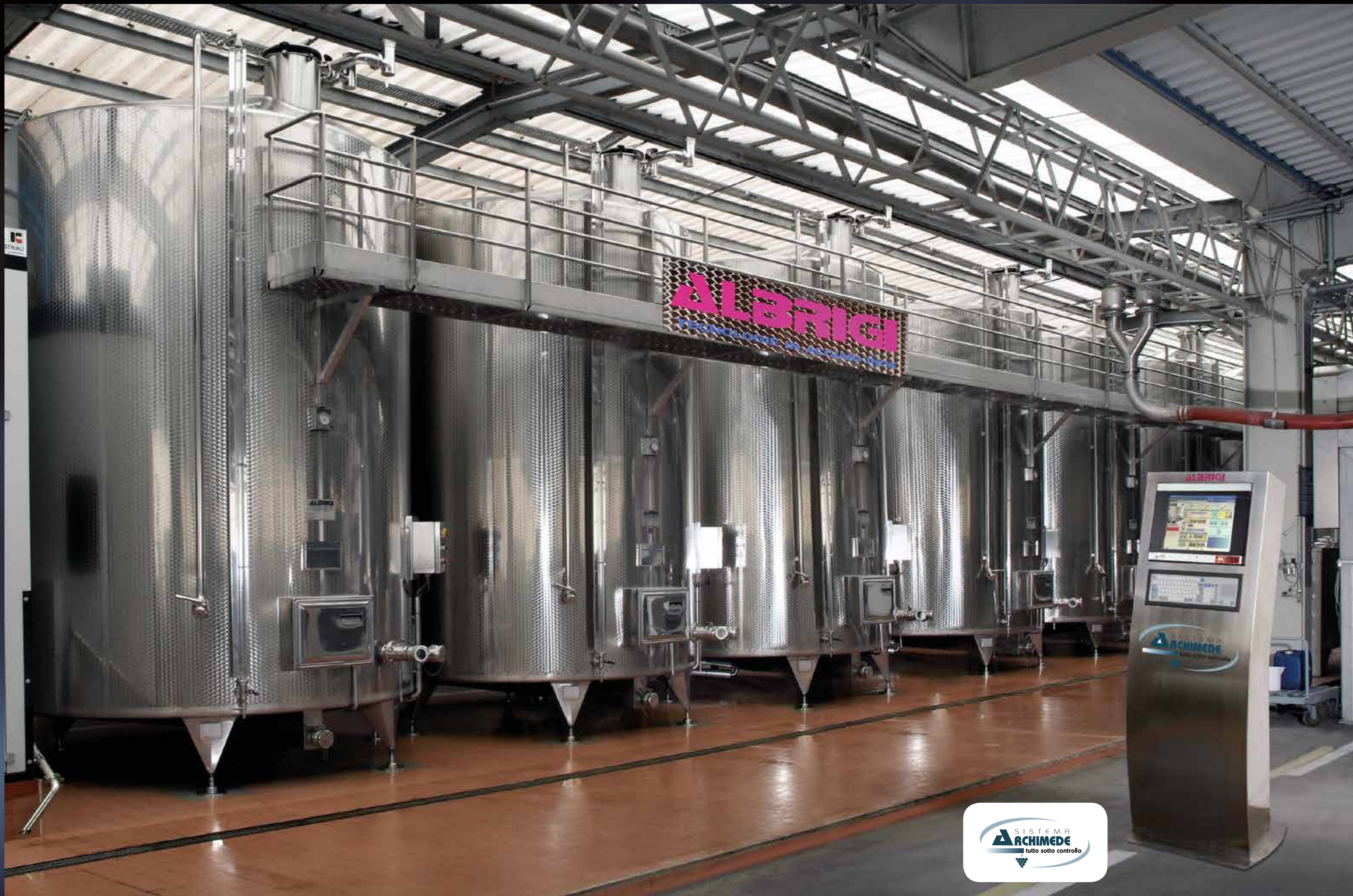
300 hl Frigitank, temperature controlled by Termostar, fitted with Isotank insulation, Sidemix stirrer and Cleanfix washing plant
