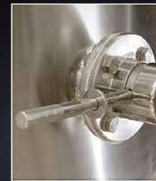
Outside view of stainless steel racking decanting arm
