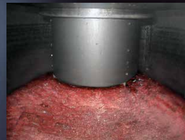
Cascade valve open showing a flow of falling must
