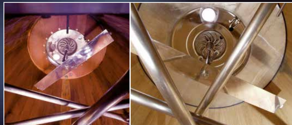
View from inside the wooden vats with patented self-rotating blade and cap-breaking poles for punching down and délestage
