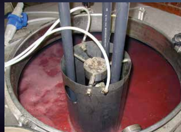
Upper compartment being oxygenized
