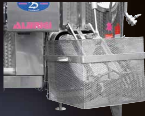
Personnel protection cage during marc discharge
