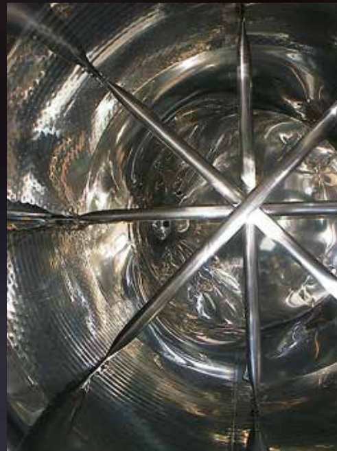
Palitank for délestage and to break up the cap during fermentation and also a help when draining off marc at the end of the fermentation
