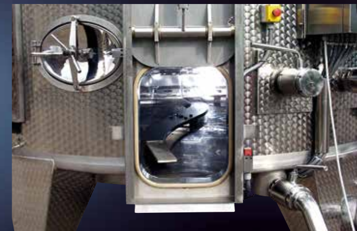
Guillotine door with "Meccanotank" mechanical marc discharge mechanism
