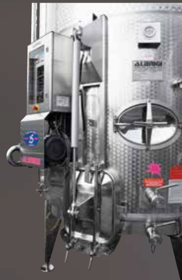
Pump for filling the upper compartment with oxygenizer and electric control board
