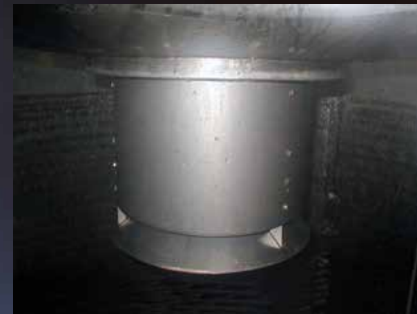
View from below of the cascade valve with the conveyor closed
