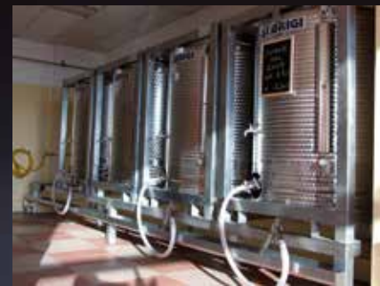
Fixed plenum unit with Innergas to serve several tanks, working with nitrogen or CO 2 with delivery rates from 20 to 100 m 3 /h
