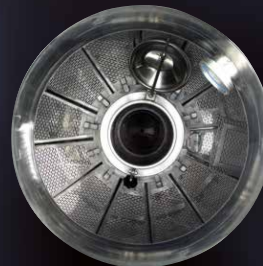
Natural must pumping over takes place with the hatchway open. Forced recirculation takes place with the hatchway closed, using the pump and the pump over tube
