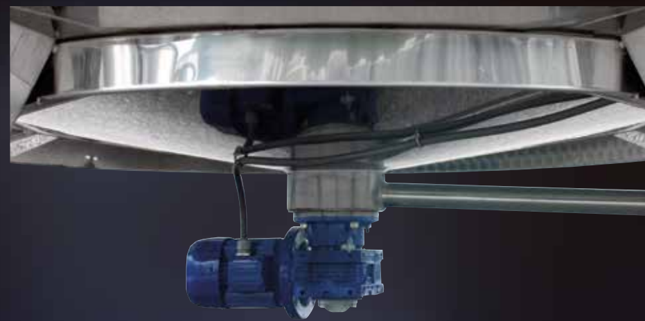
Motor to power blade rotation on the bottom
