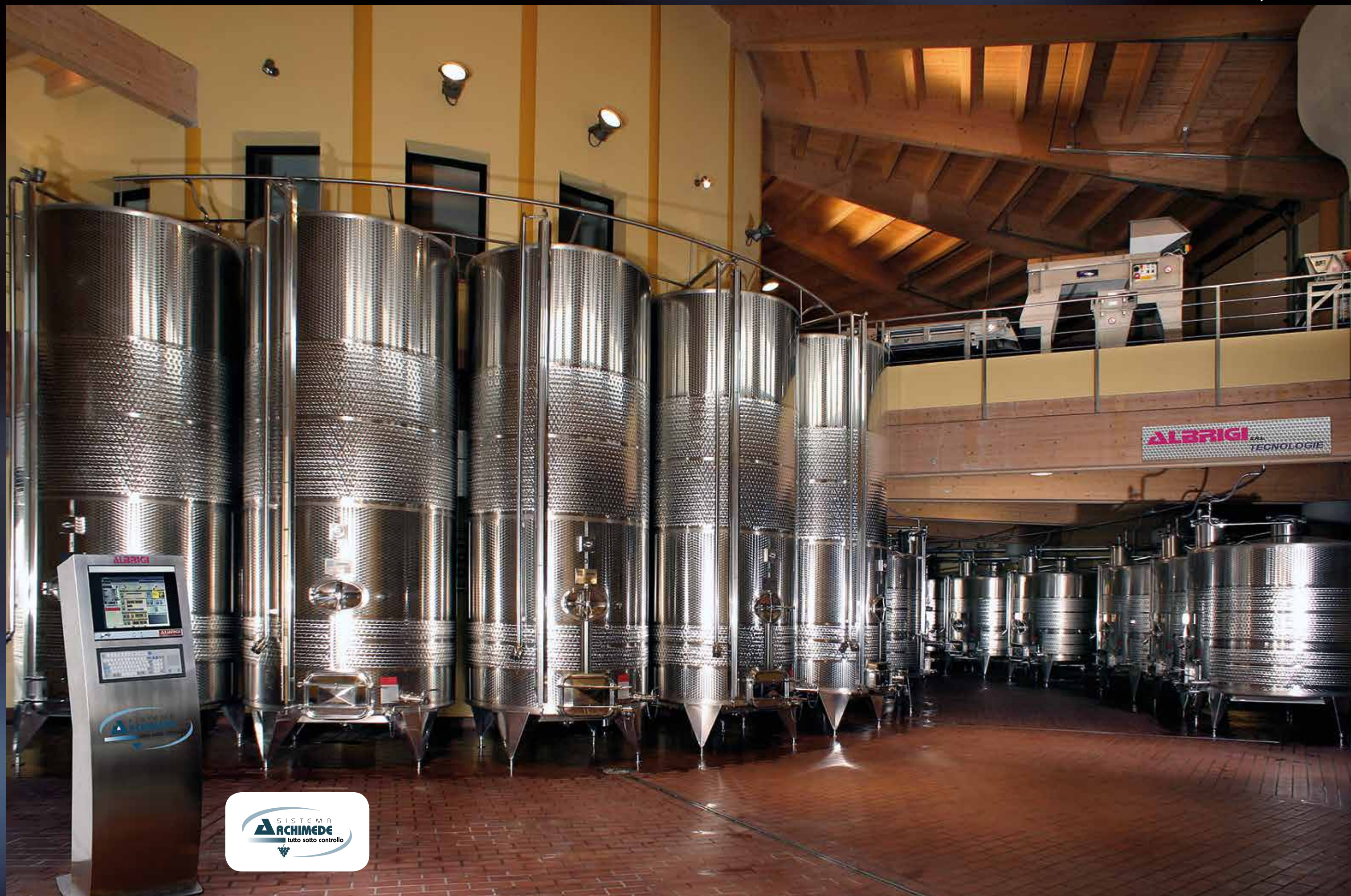
Specialtank, temperature controlled by Termostar Double, fitted with Cleanfix washing plant and Innergas system all controlled by Archimede
