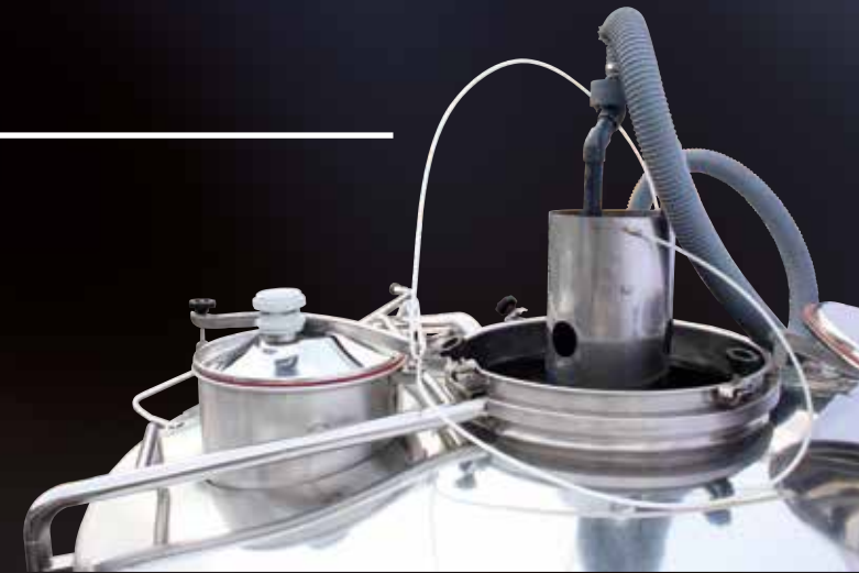
Cascade valve installed with pneumatic control system
