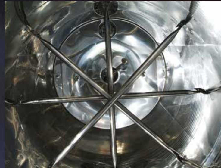
Palitank cap breaking mechanism
