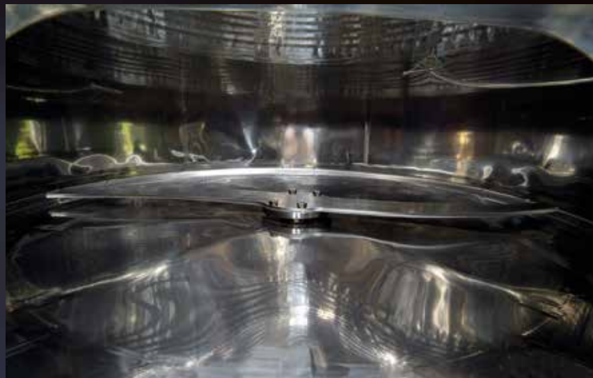
Mechanism for removing the marc from the flat bottom inclined 3% forward
