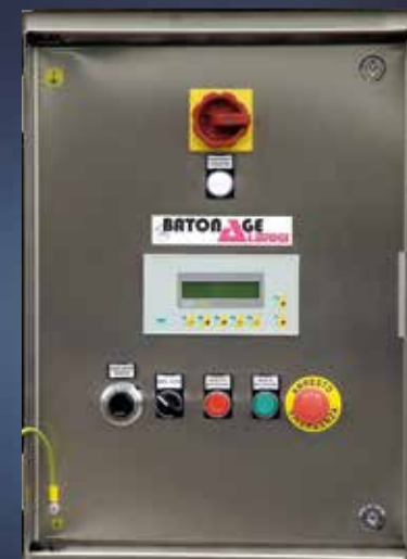
Electric Board complete with PLC and client programmed rotation cycles
