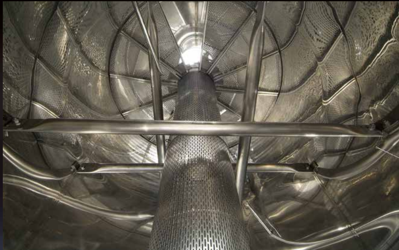
View from below of the submerged cap mechanism with cap-breaking poles
