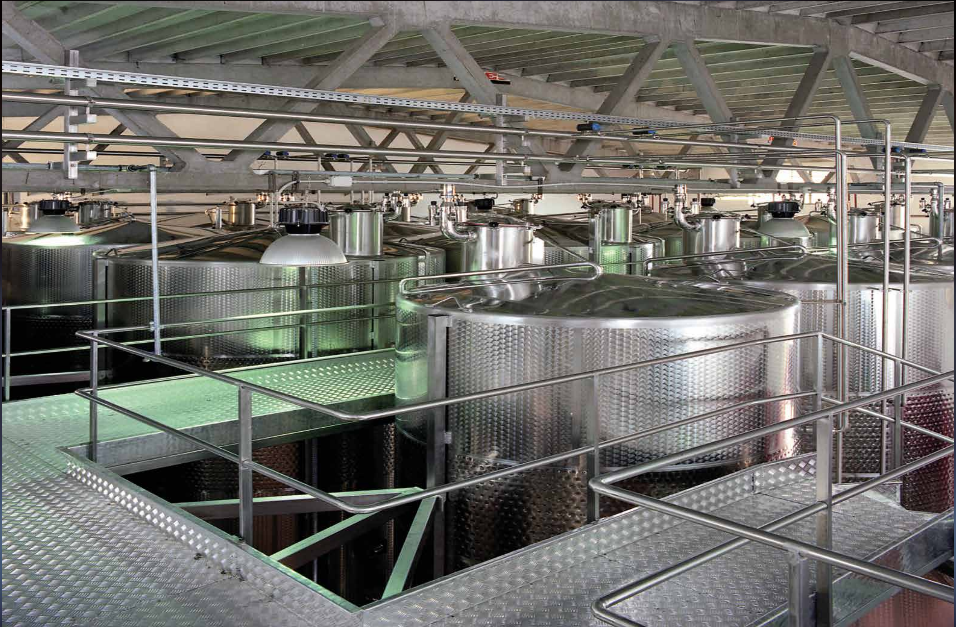
300 and 150 hl Termotanks with Innergas system and Cleanfix washing plant
