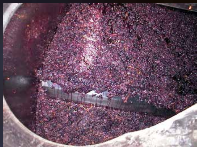
Albrigi patented self-cleaning punching down blade that plunges into the marc
