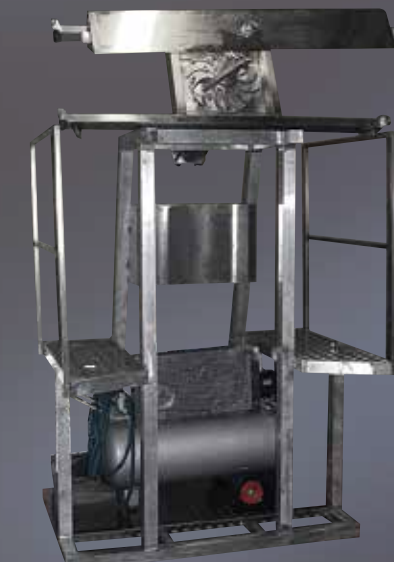
Mechanism on a mobile base for punching down with a self-rotating blade on "Vario tank"
