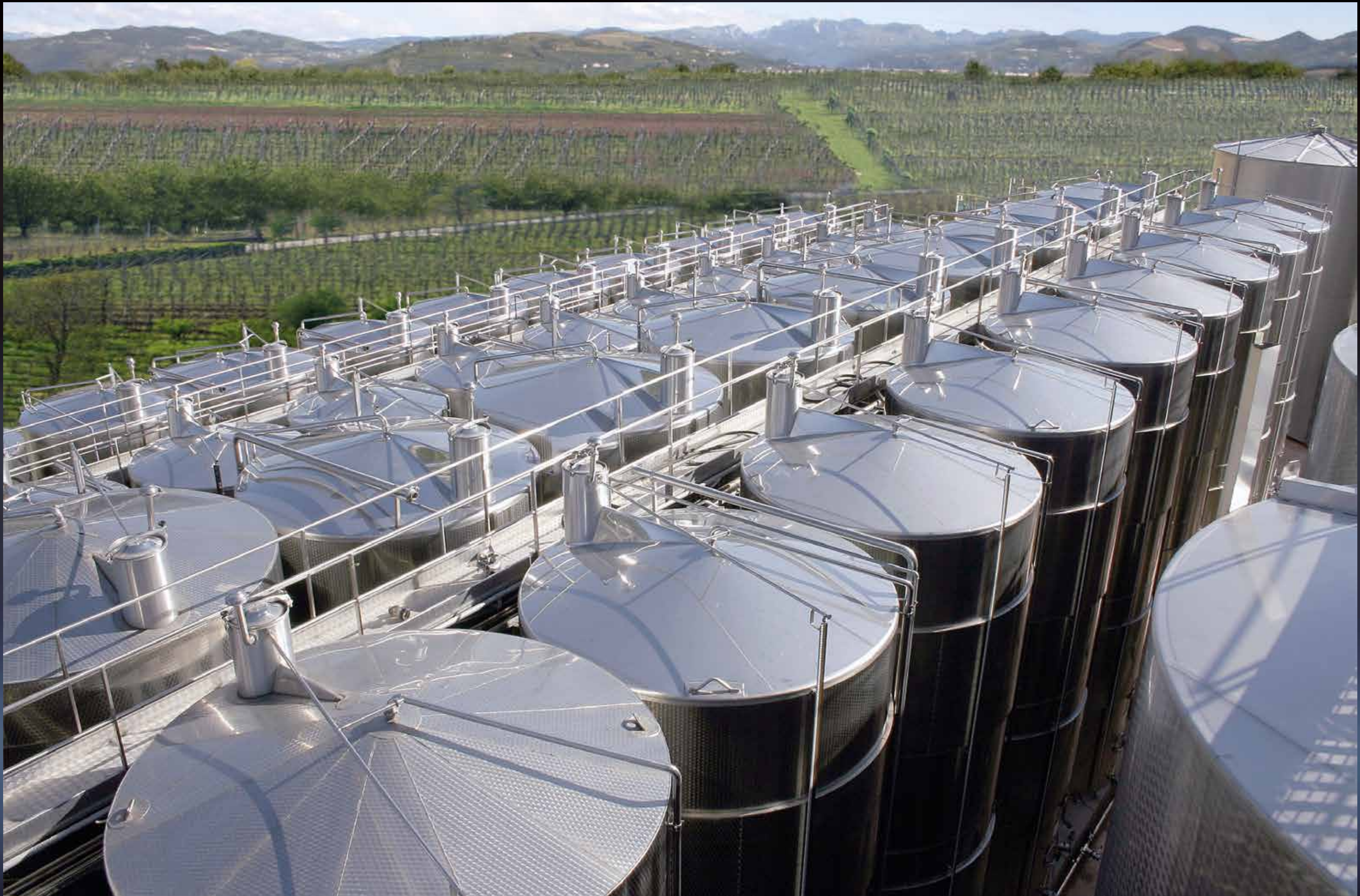
Bank of 600 hl Megatanks with 300 hl Bigtanks temperature controlled by Termostar Double and fitted with Cleanfix washing plant
