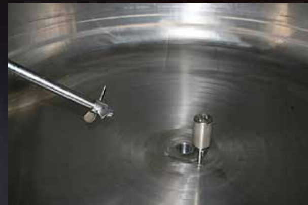
Aisi 316L sintered stainless steel porous core for sparkling process
