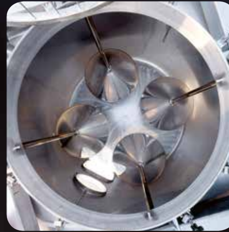
View from above of the self-cleaning punching down foot
