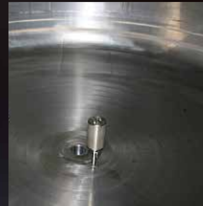
Sintered AISI 316 porous core placed on the bottom and used to introduce CO 2 from below
