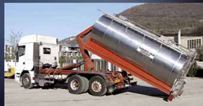
Droptank 15,000 liter roll-off insulated foodstuff tank
