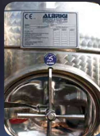
Stainless steel PED test certification plate
