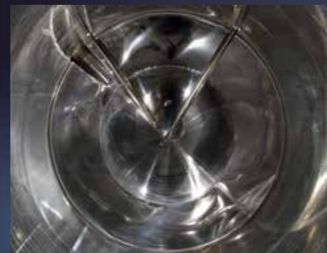
View from below of the Albrigi patented Superbottom with manhole cover air vent channels
