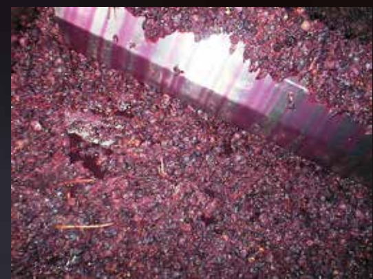
Self-cleaning Variofolltank blade
