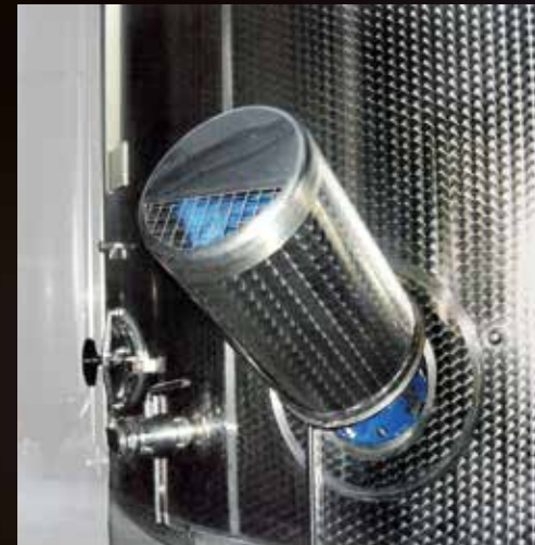
Sidemix stirrer with protective casing
