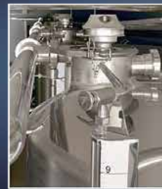
Stainless steel upper manways with vent valve
