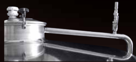
Both manual and motorized oxygenization system
