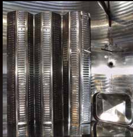
Set of 250x1000 mm mobile drainage grates to stop the skins during delestage
