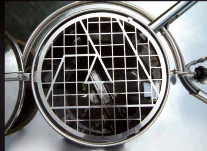
Upper manhole with protective grate and safety microswitch
