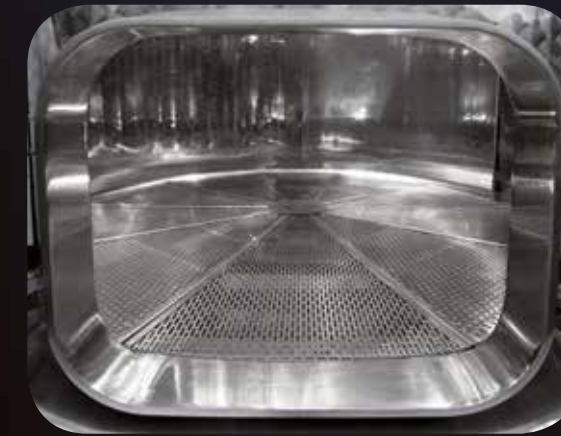
Mobile grate on the bottom to separate the grapes and drain the must
