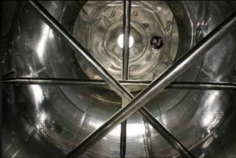
Palitank to break up the cap during délestage
