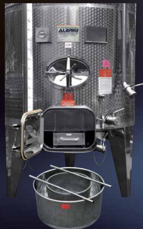
View of the lower marc discharge hatchway with the mechanism for separating the must from the skins
