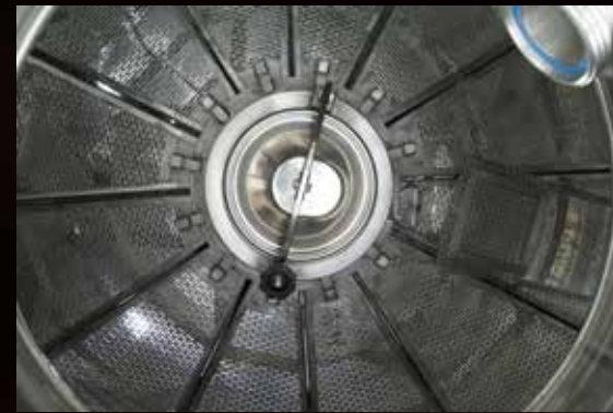
Top view of the fermenting must pressure relief hatchway
