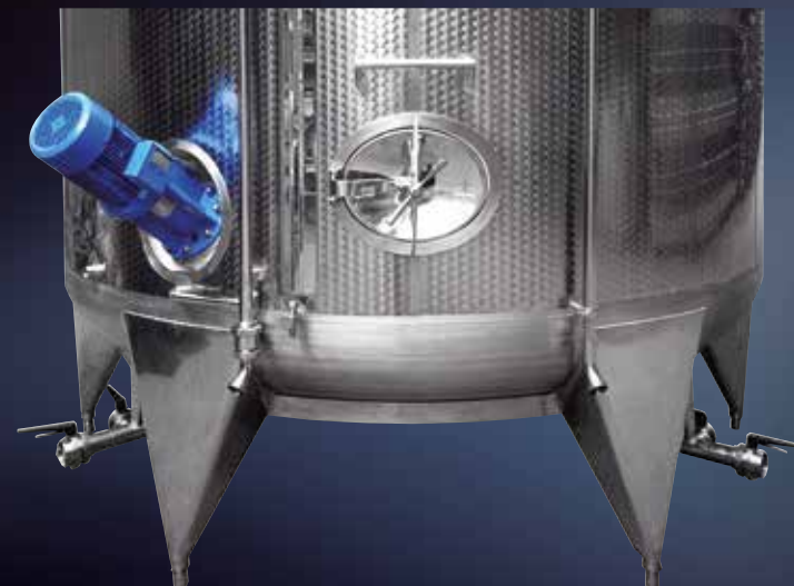
Cleanfix fixed washing plant for washing inside the Sidemix side stirrer
