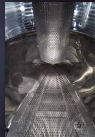
System for fastening the central fermentation pressure relief pipe to the bottom
