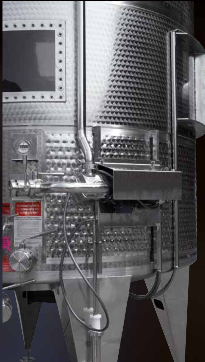
View of the pump over pump, oxygenizer and PYREX inside inspection window
