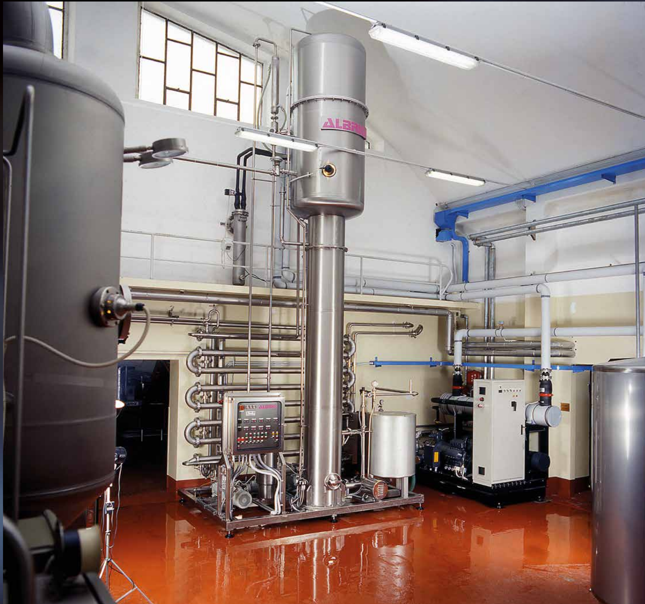
Vacuum must concentrator that works at 18/20° C for 500 liters evaporated every hour
