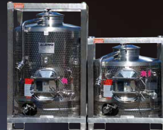
610 liter and 1070 liter Enopallet tank for micro-fermentations
