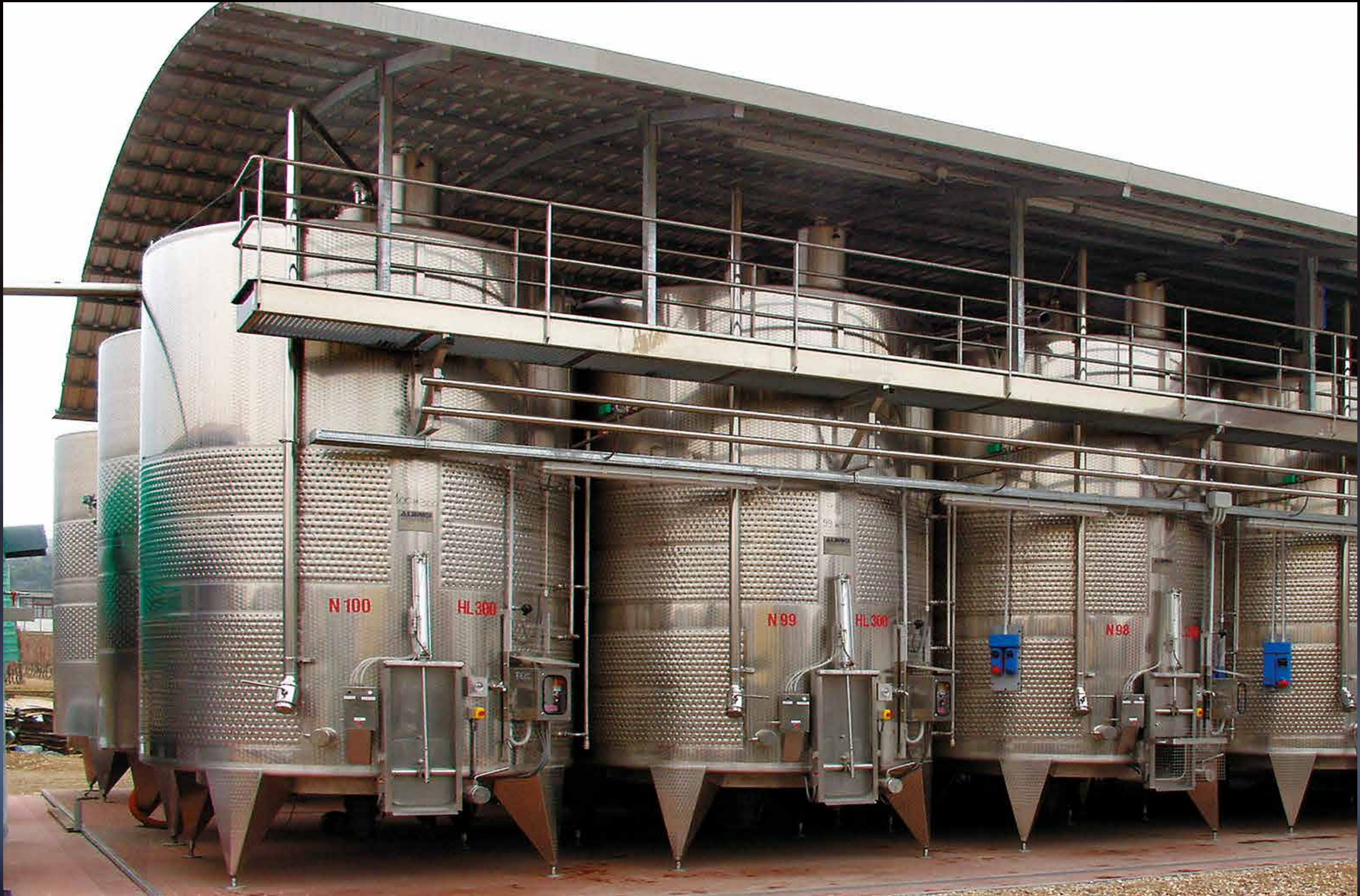
Meccanotank 300 hl fermentation tanks, temperature-controlled by Termostar Double with Palitank for délestage
