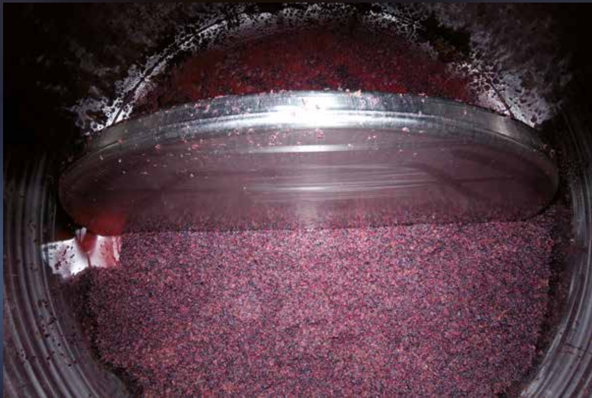
Vertically positioned rotating blade patented by Albrigi, with dry-raisin marc during a pause in the work cycle
