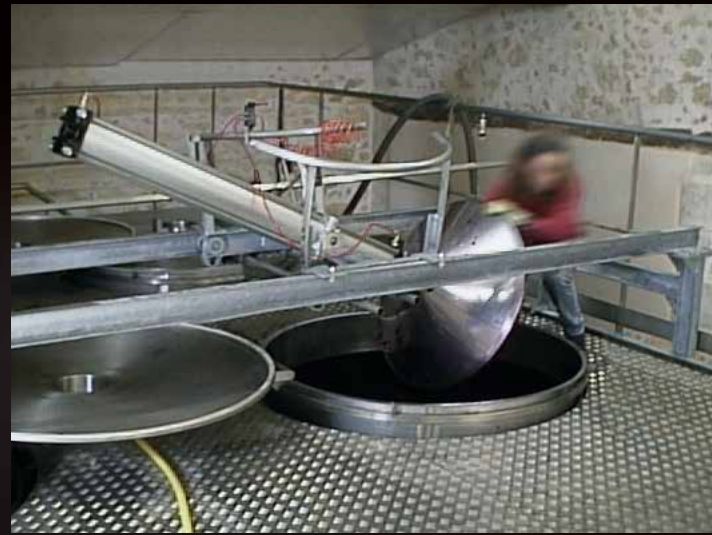
Using and adjusting the Albrigi patented self-cleaning single-foot punching down mechanism
