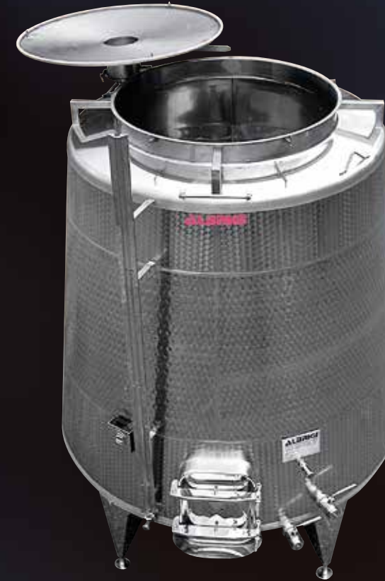
Large manhole cover for punching down
