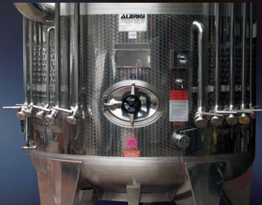
Service valves for the upper compartments of a three-compartment Politank with total and partial drain, washing, nitrogen and pumping over systems
