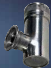
Stainless steel dia. 40-50-60-80 mm demountable double-acting valve with weighted overpressure and vacuum plates with anti-adhesive viton and teflon "O-ring" seals
