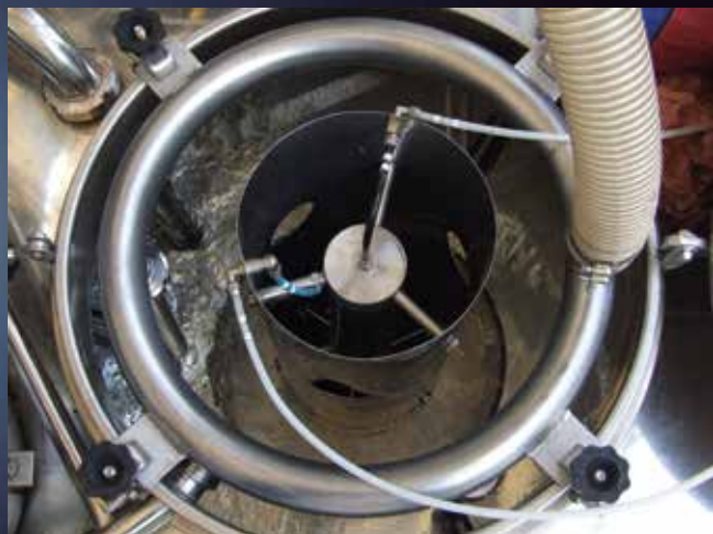
Cascade valve with air injector
