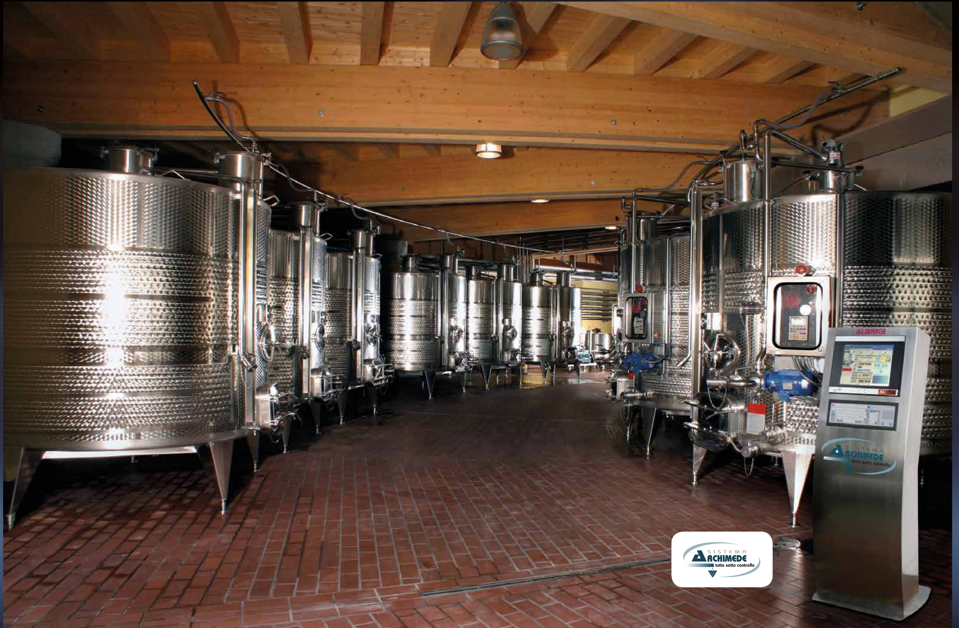
Meccanotank winemaking tanks, temperature controlled by Termostar Double and fitted with Cleanfix washing plant, Innergas system and Motorfly pumpover
