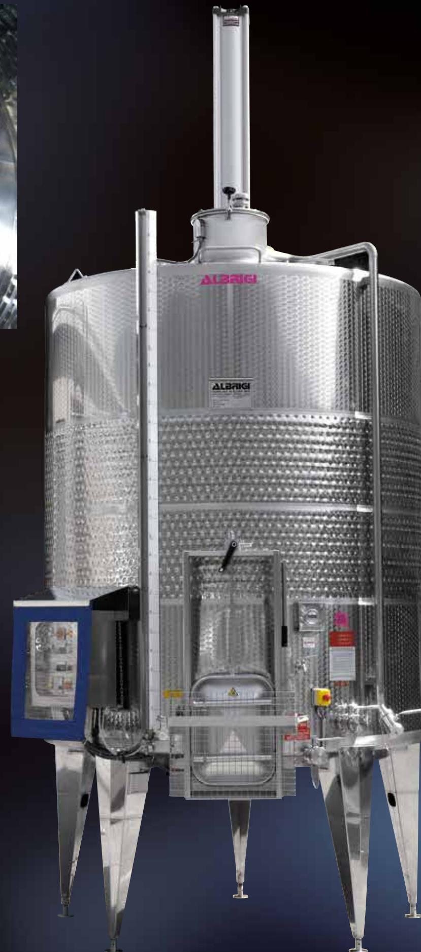
100 hl Monofolltank temperature-controlled fermentation tank with punching down mechanism that can be removed and stored at the end of fermentation, turning the fermentation tank into a standard wine storage tank
