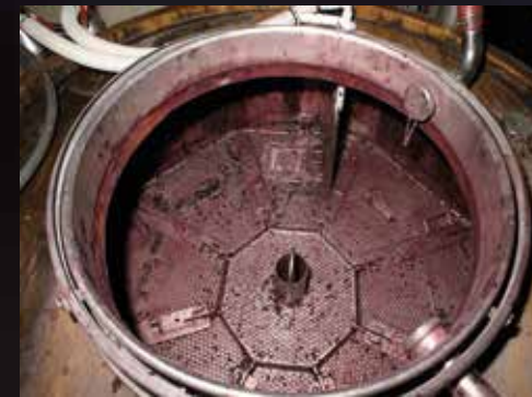
Submerged cap mechanism on a wooden vat, removable from the outside
