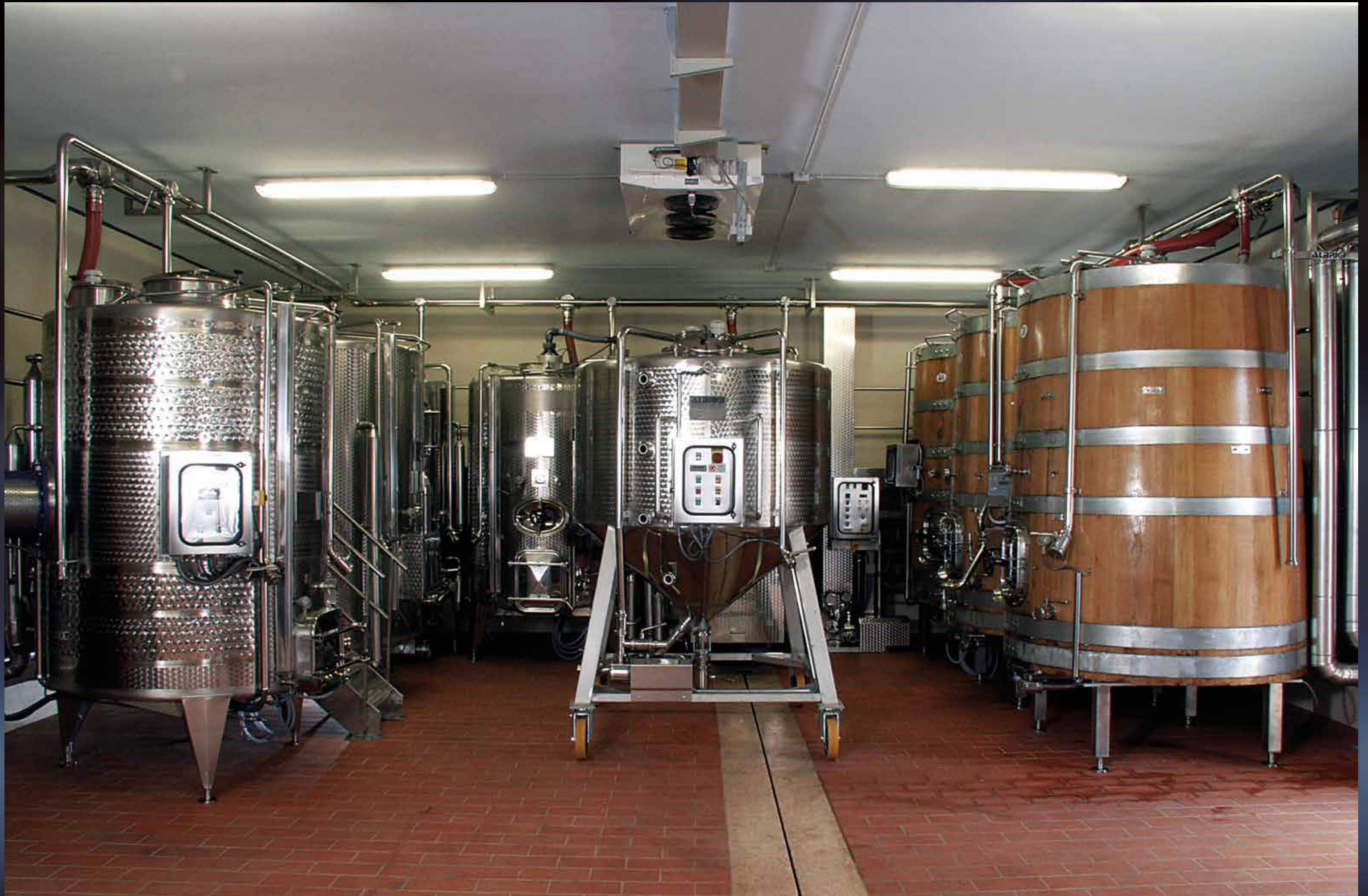
Bâtonnage - Délestage - Spartank - Volvotank - Frigotank - Noveltank - Pluviatank - Criotank – Monofolltank - Supertank Experimental fermentation cellar with 9 different types of fermentation tanks and a static grape seed separator
