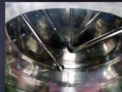
Albrigi patented Superbottom bottom and counter-bottom with Sprayball washing ball
