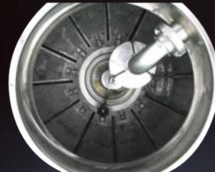
Disk for flooding must over the submerged cap mechanism
