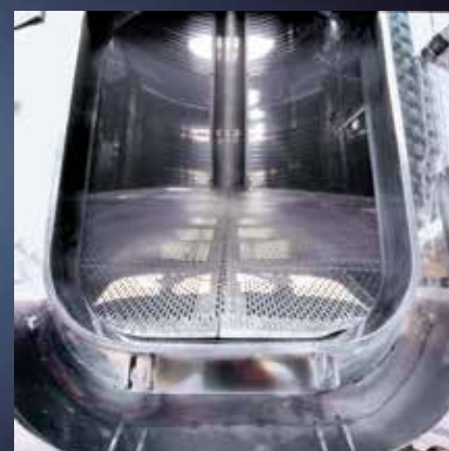
Demountable grate, removable through the hatchway
