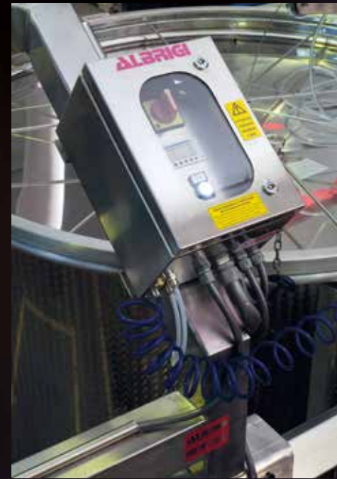
Electropneumatic control board for manual/automatic lift and lowering
