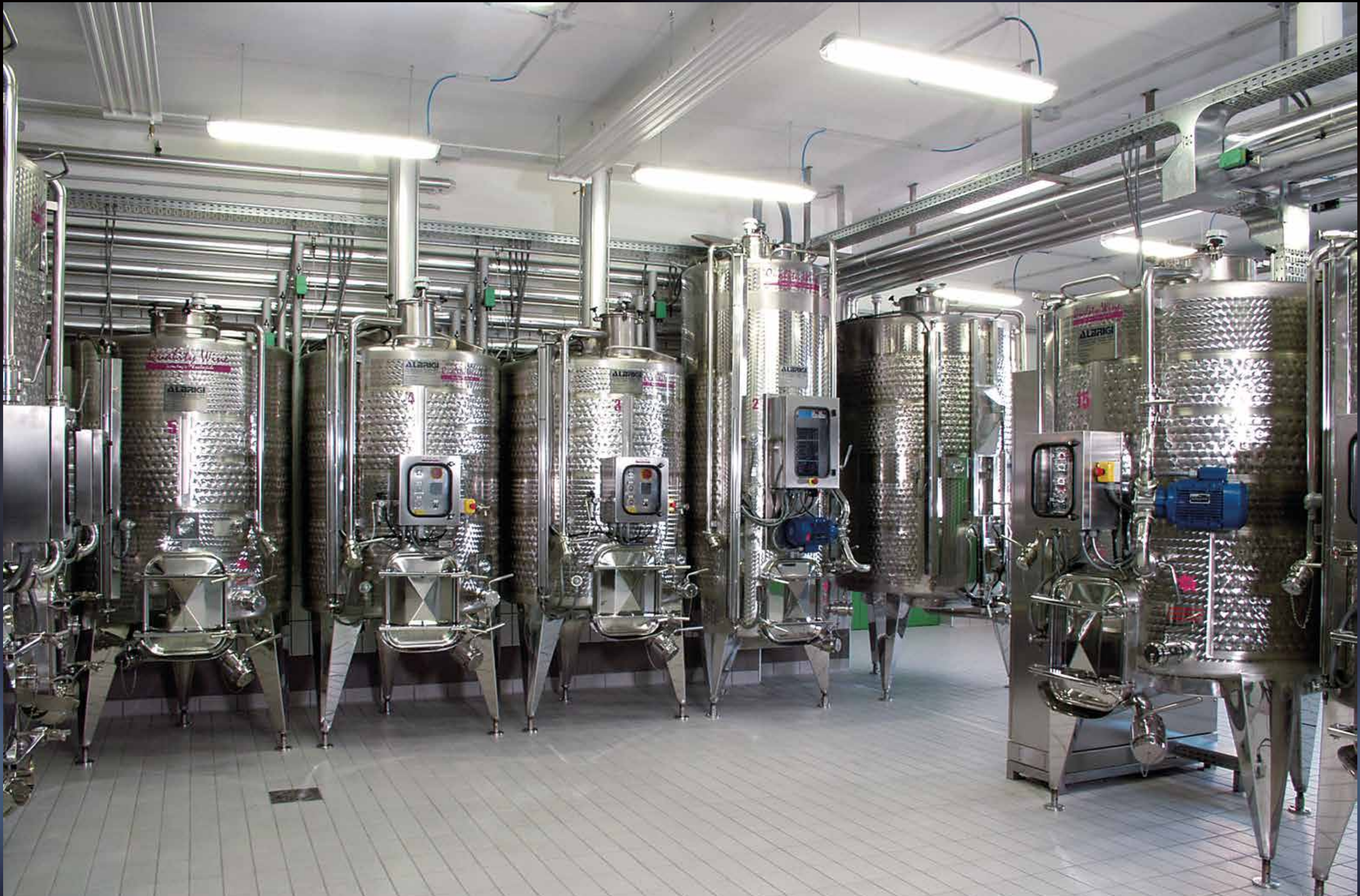
Set of fermentation tanks - Délestage - Monofoltank - Supertank – Pluviatank, temperature-controlled by Termostar equipped with all accessories
