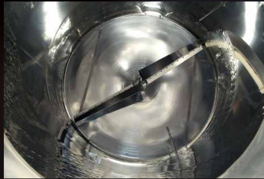
View of the patented rotating blade on the bottom.
