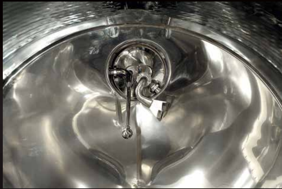
Inside view of the self-rotating must sprayer and the washing ball
