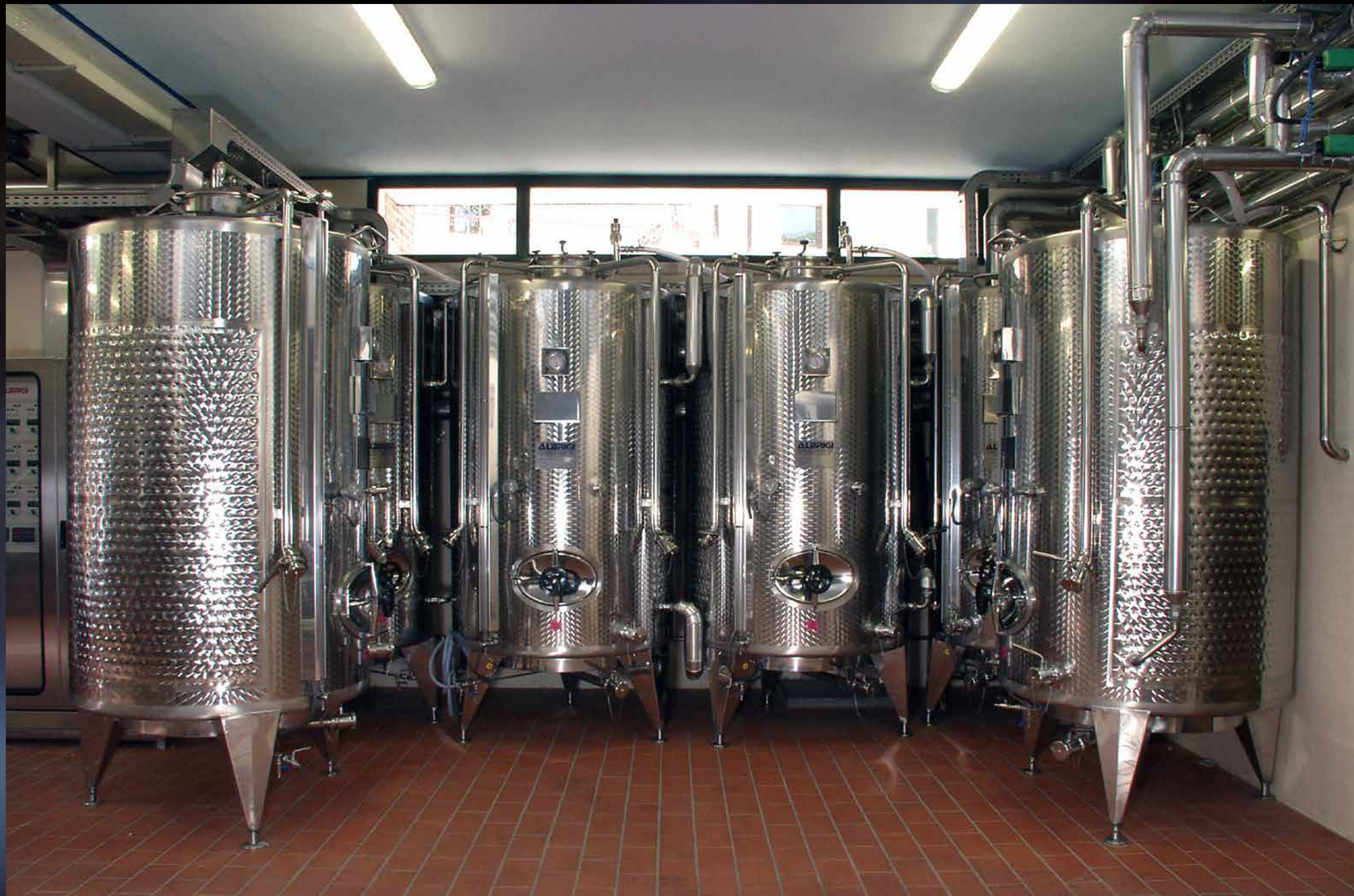
Storage department with tanks with Termostar jackets for malolactic fermentation with Innergas
