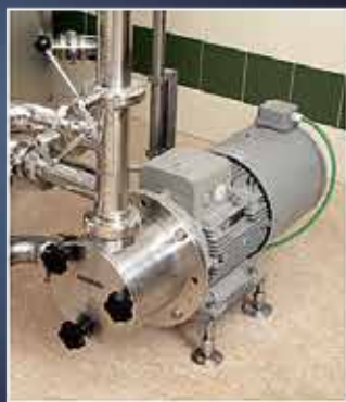
Stainless steel low-speed pump
