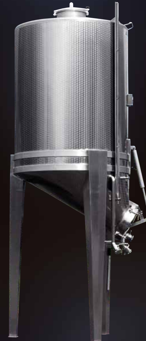
The offset truncated cone bottom favors gravity drainage of the marc
