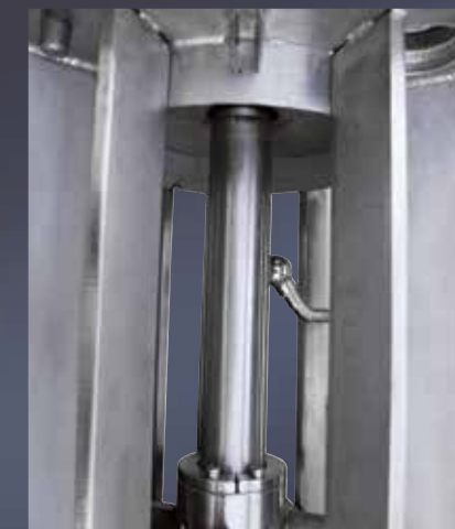
View from above of the must outlet baffles with the anti-vortex propeller and washing plant
