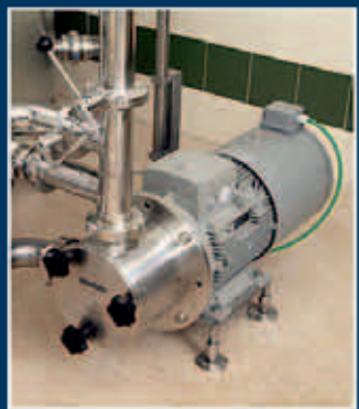
Pompa inox lenta Stainless steel low-speed pump
