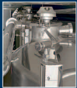
Chiusini con sfiato aria Stainless steel upper manways with vent valve
