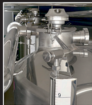
Manhole cover with air valve
