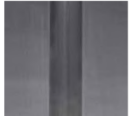
Rolled and mirror polished interior Tig/plasma welding on mirror polished sheet metal 2R finish 0.06 Micron roughness
